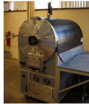
Figure 2. Microwave furnace for sintering and reactive sintering of CNT loaded composite materials.
